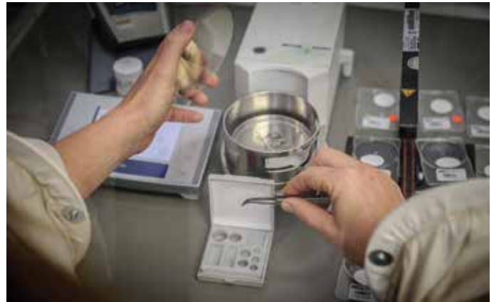
Exercising and intermediate check of the performance of the microbalance with the calibrated mass pieces prior to weighing the filters Photograph: BBE Laboratory
