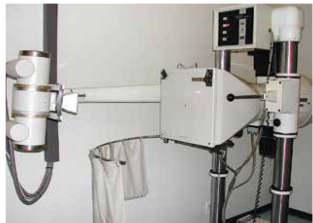
A mass miniature radiography (MMR) machine
