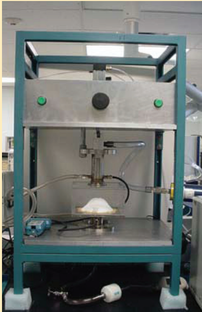
Figure 12. A flat plate test system for measuring respirator filter penetration of 3 to 20 nm silver particles
