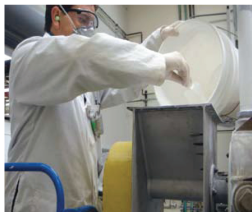
Figure 11. A nanoparticle production worker wearing a personal air sampler and hearing, respiratory, and dermal protection during a pouring operation
