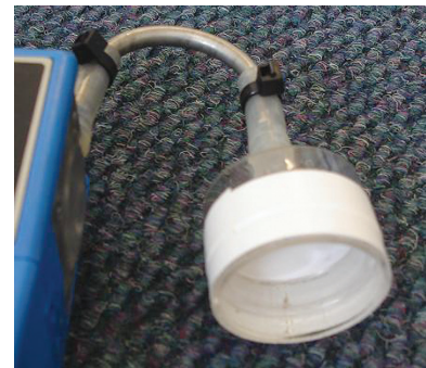
Figure 3. Open face DPM sampling method
