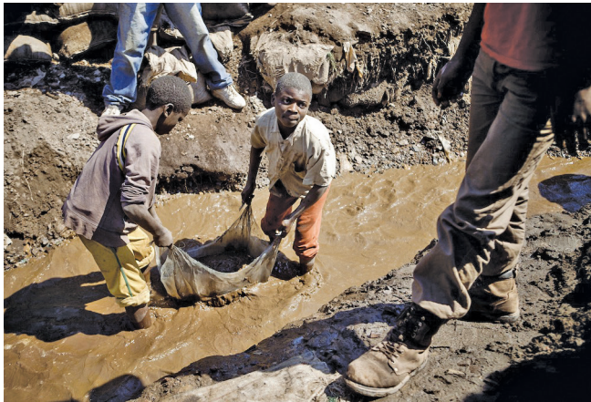
Children washing and sorting copper ore in water and mud, at an open-air mine in Kamatanda in Katanga, southeastern Democratic Republic of the Congo
